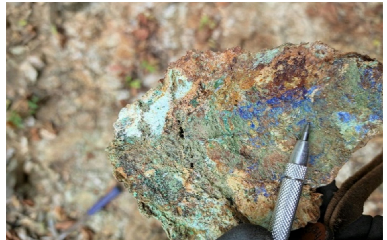
Figure 5: Hand specimen displaying azurite and malachite copper oxide mineralisation taken from the Copper Ridge prospect, Linderos Project
