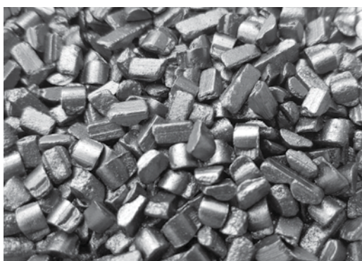
Figure 12: High quality, low impurity Balama natural graphite recarburiser (each approximately 5mm long)
