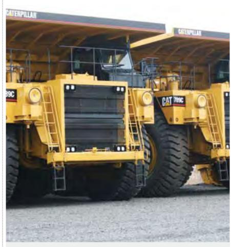
One of the features of Ferrexpo's drive to reduce costs and increase operating efficiencies is the application of innovative solutions to mining operations. A good example is the direct loading of CAT 789 haul trucks by dragline to avoid costly re-handling. The draglines manufactured locally by NKMZ, which appeared in the 2008 Procurement Case Study, are now in operation at the new Yeristovskoye mine.
