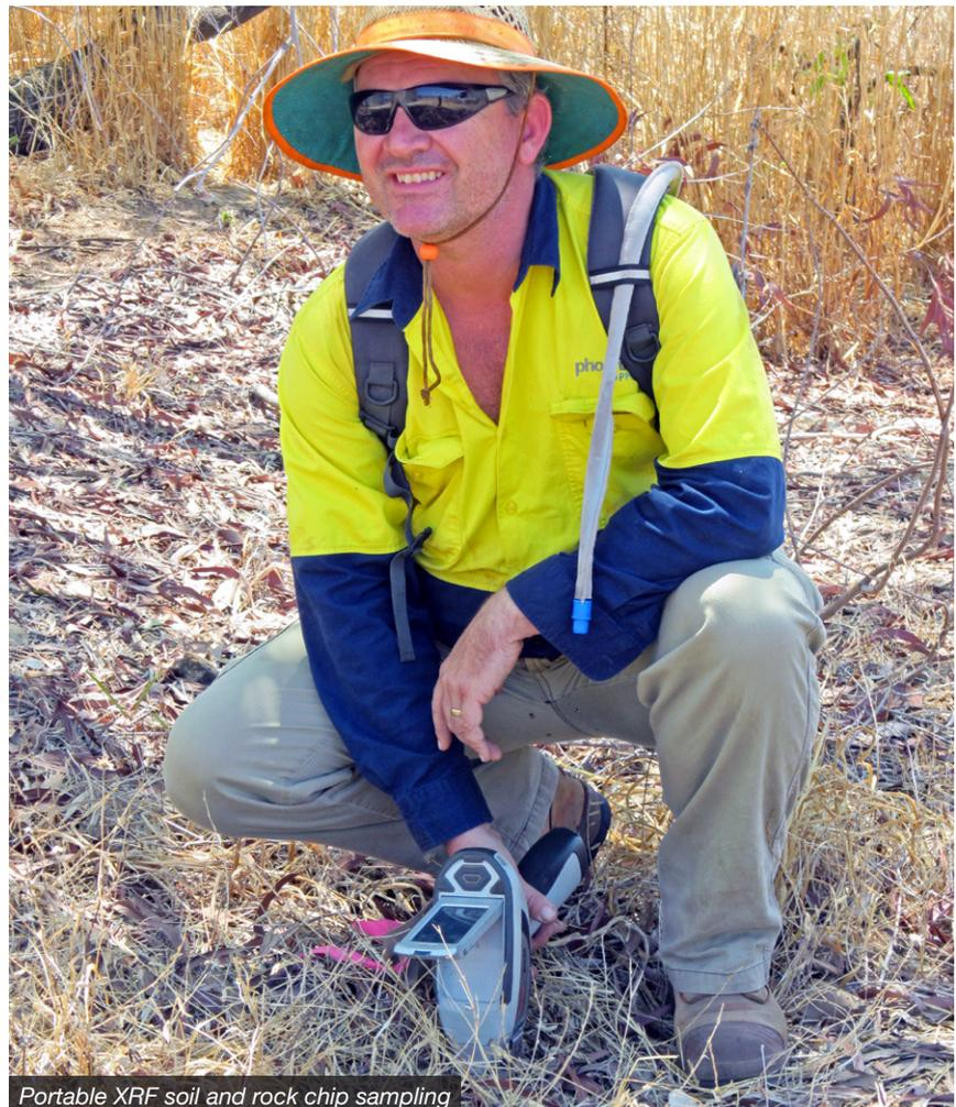
Portable XRF soil and rock chip sampling
