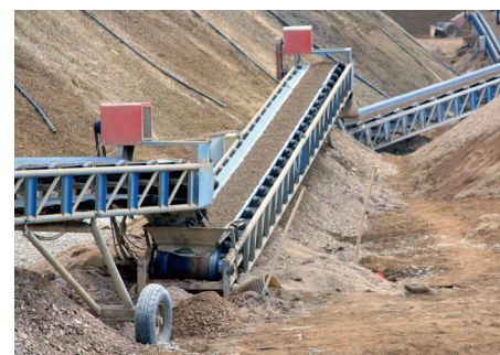
Ore conveyance to leach pads
