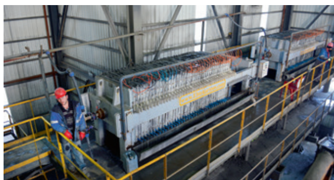
The two filter presses which are used to produce the final concentrate.
