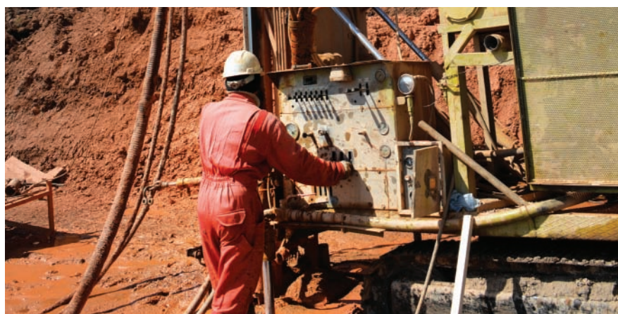
Reverse circulation drilling at the Ugur deposit.
