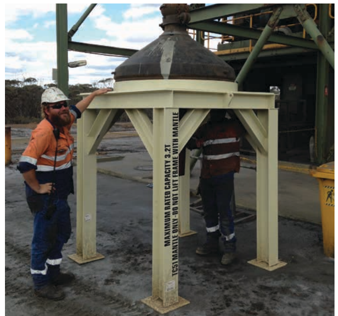
Maintenance Technicians Luke Hamon & Rob Watts testing the new Crusher Mantle Maintenance Frame
