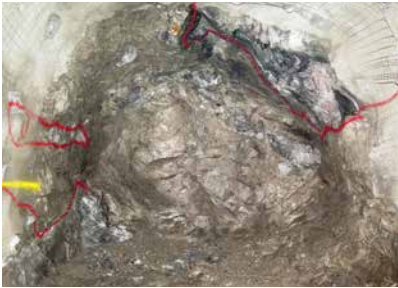
FLYING FOX ORE DRIVE WITH AN AVERAGE GRADE OF 8.3% NICKEL.
