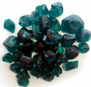
HIGH GRADE NICKEL SULPHIDE PRECIPITATE AND NICKEL SULPHATE CRYSTALS
