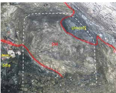
SPOTTED QUOLL ORE FACE WITH AN AVERAGE FACE GRADE OF 8.5% NICKEL
