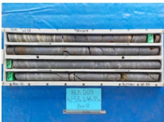
Figure 6: BEKD09 – Massive iron mineralisation from 42.8m to 48.0m within a zone of more lenticular magnetite mineralisation, start and end shown within the yellow arrows.
