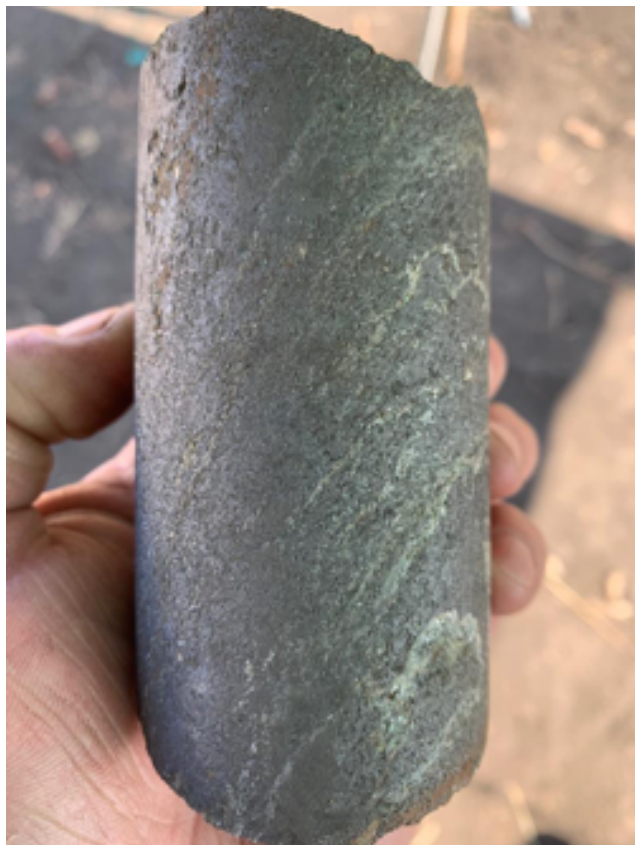
Figure 6: BEKD09 – Massive iron mineralisation from 42.8m to 48.0m within a zone of more lenticular magnetite mineralisation, start and end shown within the yellow arrows.
