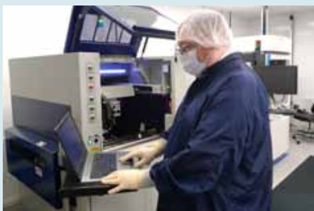
Automated bonding and assembly of CZT detector modules
