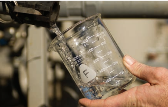
Here, a water sample is drawn for testing. Devon is using recycled water in the Barnett Shale to reduce consumption of fresh water.
