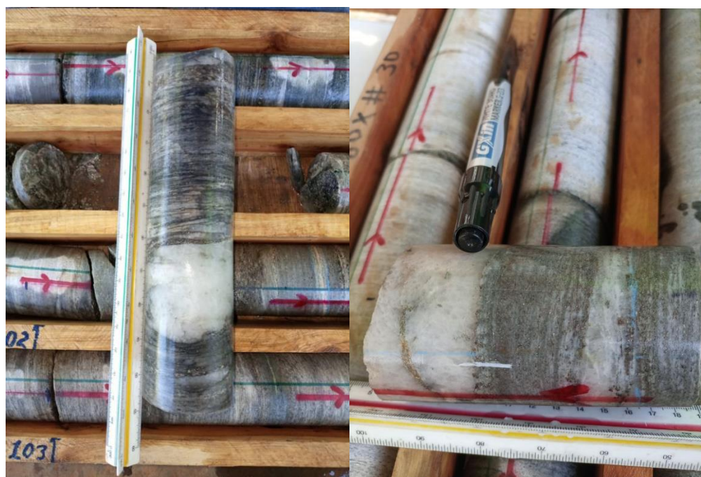
Figure 5: Drill core from Hole 1 (BBDD001), showing intervals of highly altered host rocks and quartz veining, both with significant visible sulphide mineralisation (pyrite, chalcopyrite, pyrrhotite). Left: ca. 101m Right: ca. 106m
