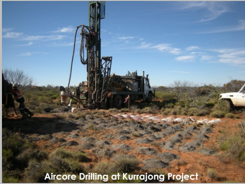
Aircore Drilling at Kurrajong Project
