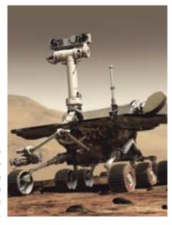
Spirit and Opportunity rovers exceeded their planned life span, sending images of Mars to Earth using Ball antennas and electronics.
