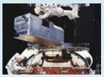
Ball-built Corrective Optics Space Telescope Axial Replacement (COSTAR) installed on Hubble Space Telescope, fixes Hubble's blurred vision, 1993
