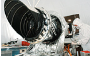
The HiRISE camera, launched in August aboard the Mars Reconnaissance Orbiter, will take the most detailed images of Mars ever sent from an orbiting spacecraft.
