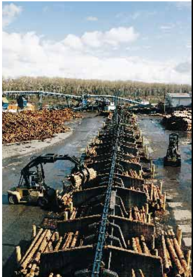
Scandlog short-wood log handlers sort and store logs at Interfor's Western Whitewood sawmill near New Westminster, British Columbia.
