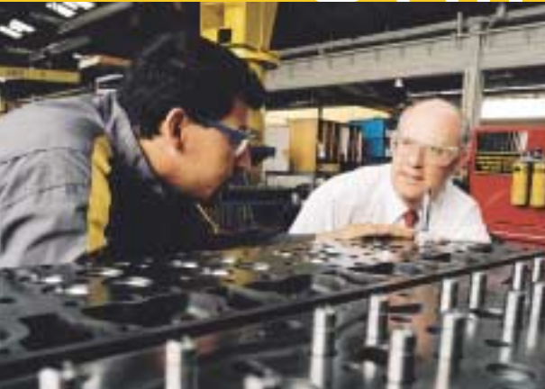
Nick Lloyd (right) watches as mechanic Daniel Bravo checks on newly inserted valve guides on a Caterpillar engine in Finning Chile's Santiago service department.
