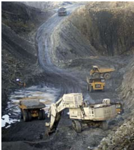
Oxide ore is trucked from the Plant-North pit to Bogoso where it is crushed and then ground in the mills in the foreground, at right. A ramp extending underground from the bottom of the pit could access the near-surface mineralization in the inactive Prestea Underground Mine.
