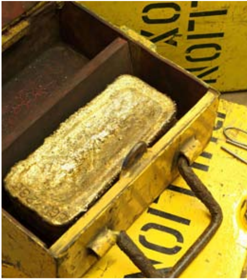
This doré bar at our Bogoso plant is approximately 90% gold and contains about 450 troy ounces. It is worth $225,000 at $500 an ounce. Security is tight in the refinery!
