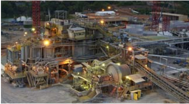
The $125 million sulfide expansion project at the Bogoso recovery plant is being constructed in parallel with the existing oxide plant. It will increase total throughput capacity from 1.5 million tonnes per year to 5.0 million tonnes.
