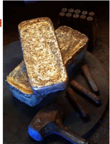
The refinery crew jokes together after a hot day's work refining gold. The doré bars are about 90% gold and are shipped to South Africa to be refined to 999.9 fine gold.
