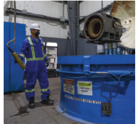
Calgary, AB: A technician preparing to complete the insulation of a rewind electric motor.
