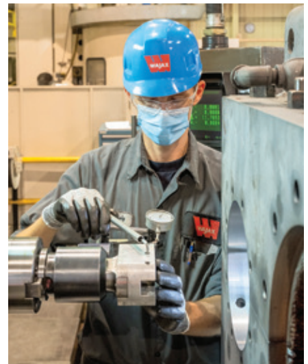
Lasalle, QC: ERS machinist setting a cutting tool prior to horizontally boring a gearbox housing.
