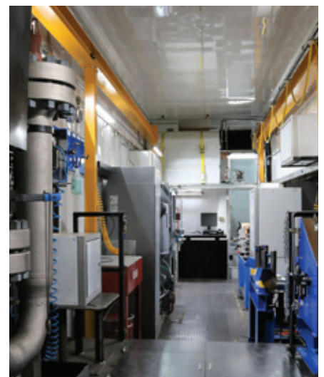
Tundra's fully equipped mobile valve service centre allows technicians to address valve service and repair needs on-site via a self-contained 53-foot trailer.
