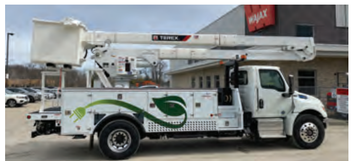
Wajax tested, stabilized, and provided training on the operations of this fully electric bucket truck.
