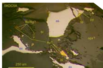
Figure 3: Fine free gold (Au) along grain boundaries at Dugbe F (qz-quartz, bi-biotite, pl-plagioclase, ap-apatite, po-pyrrhotite, as-arsenopyrite)
