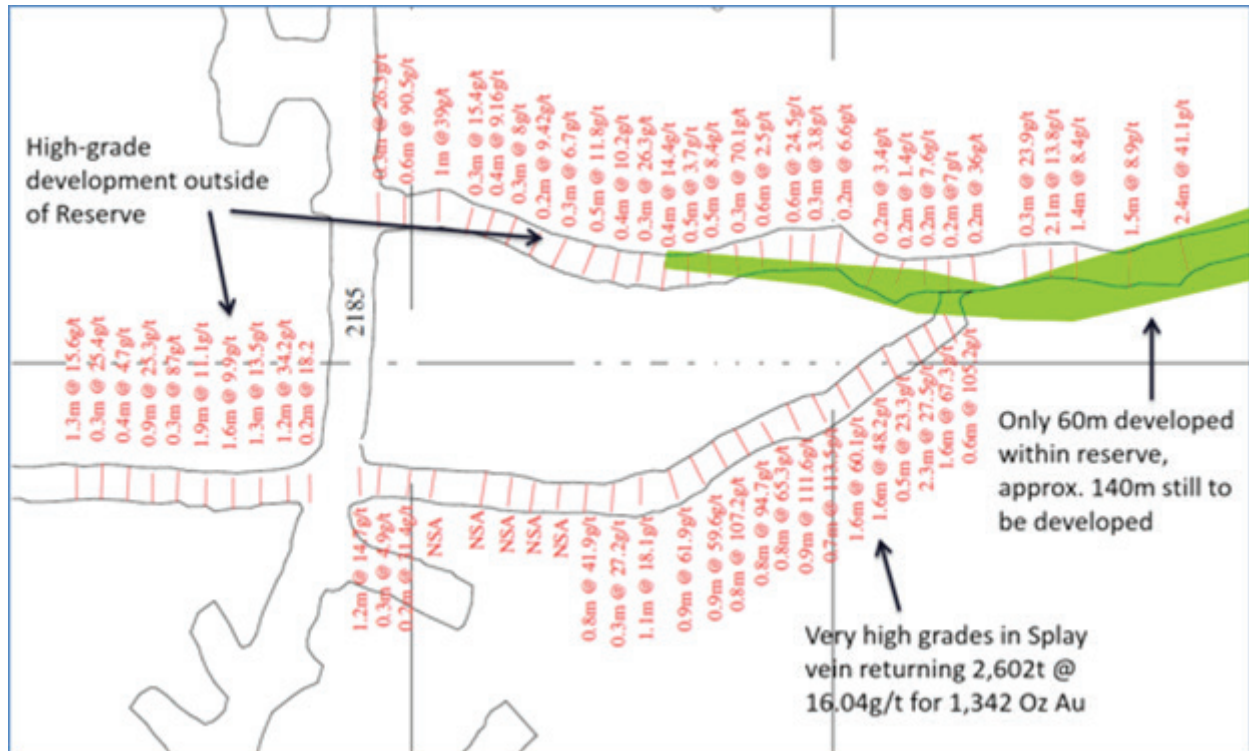
Figure 1: 2185 Level Development to end of March 2016, showing large amount of ore developed outside of reserve including very high grades in the splay vein
