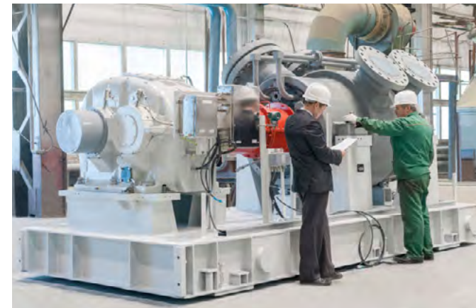
Gas compressor package on the basis of the 25MW 5GC2-287/15-57 GTU compressor
