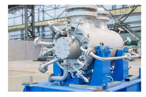
Centrifugal compressor 4GC2-75/30-83 GTU with gas-turbine engine
