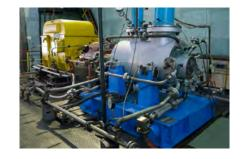
Testing of centrifugal compressor
