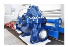
Centrifugal double suction pump type series Del ium
