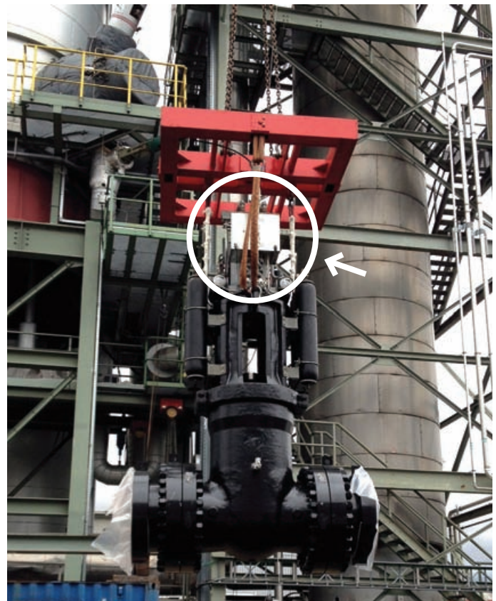
Curtiss-Wright's Electro-Hydraulic Operator (EHO) was successfully tested on a critical isolation gate valve during a high flow QME-1 testing. The critical isolation gate valve supplied for steam service requires both tremendous power and precise speed to work properly. The operator and valve had to successfully overcome more than 160 tons of thrust while the gate of the valve traveled 26" within 2 and 5 seconds.
