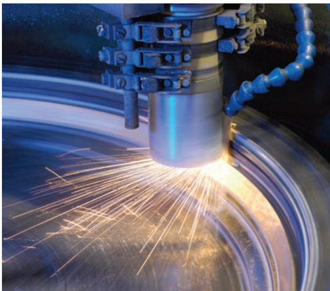
Electro chemical finish grinding of a turbine engine honeycomb seal by CCRS.
