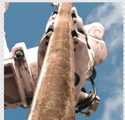
Our 4200 surface exploration drill includes a hands-free diamond rod handler, which picks up rods, makes and breaks rod joints without the need for manual operation.
