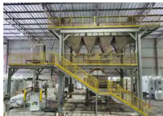
The CRF production line in Varginha, Brazil, which produces 25,000 tonnes of fertiliser annually
