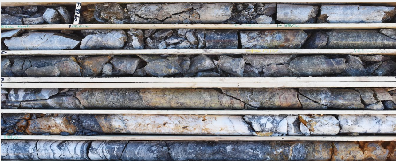
GNDD-035 (88 to 93m) - 5.75m at 9.5 g/t Au, 29 g/t Ag, 3.5 % Zn from 88.8m
