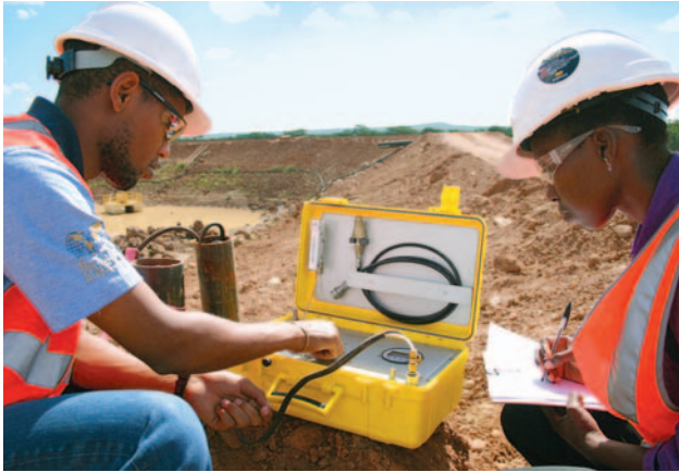
Environmental staff monitor pore pressure on the water storage dam wall at Tulawaka, our newest mine in Tanzania.
