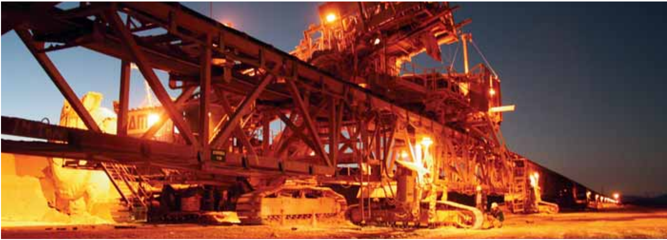
Bucket loaders at the Zaldívar copper mine remove leached material from the pad to make room for fresh ore from the conveyor.
