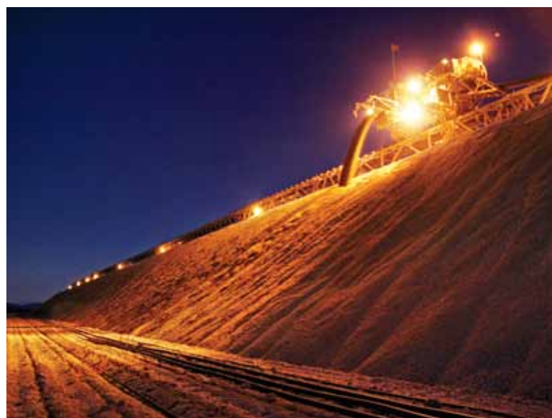
The leach pad at Zaldívar is refreshed with ore in a constant cycle of delivery and reclaim.
