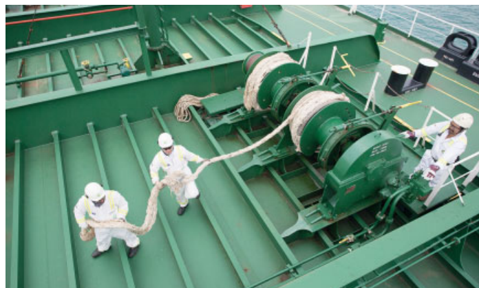
▲ Crew carrying out mooring operations on the deck of BP's oil tanker, British Chivalry , as it berths in Singapore.
