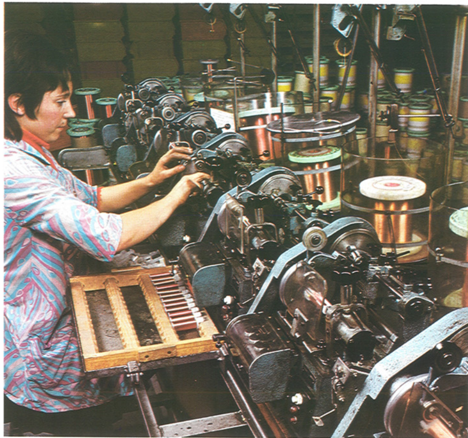
Multiple-machine system for winding relay coils in the Group's factory at Eu, France, operated by the French subsidiary, Société Française des Téléphones Ericsson.
