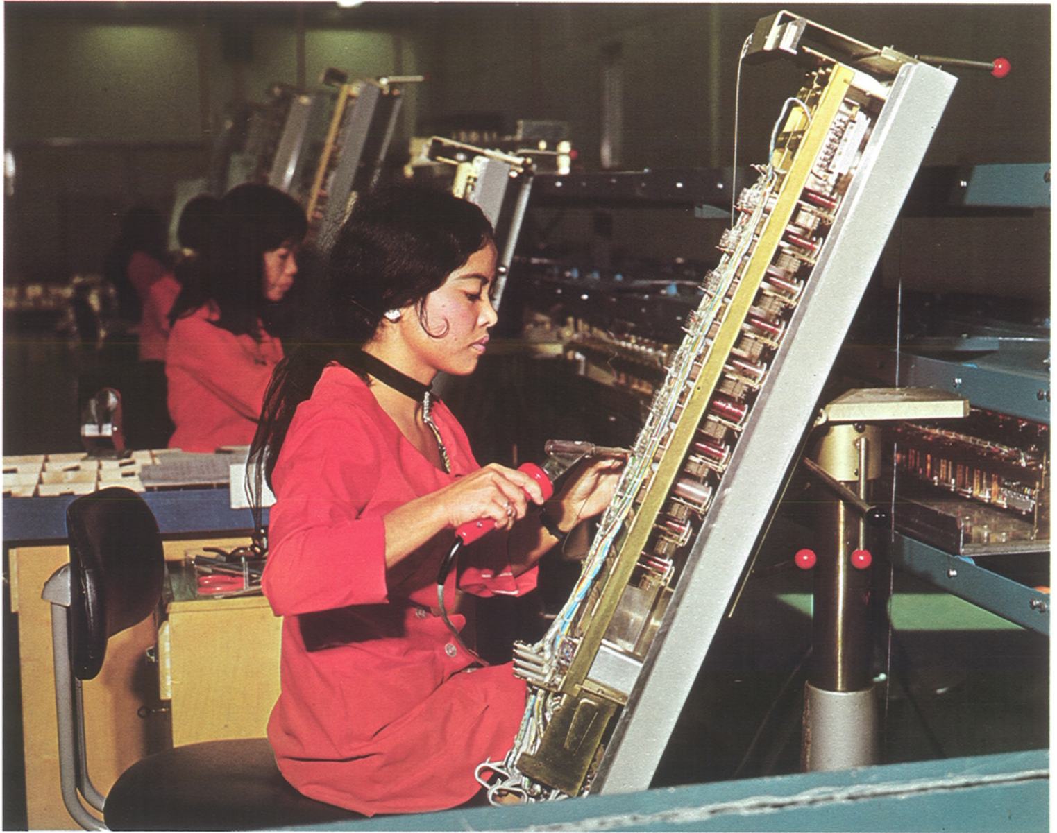
Soldering of relay racks in Ericsson's factory at Kuala Lumpur, Malaysia. The plant, inaugurated in March 1971, produces primarily automatic telephone exchanges.
