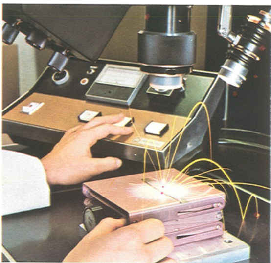
A ruby laser is used to develop new welding methods in the manufacture of mechanical components.
