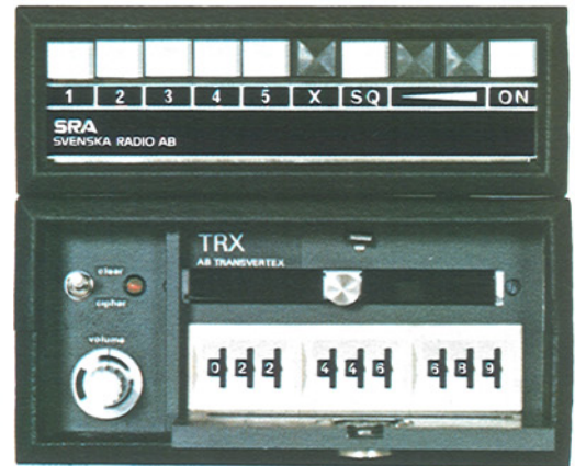
AB Transvertex produces devices to safeguard privacy in radio telephony. Unit shown here is being used with a mobile radio system developed by Svenska Radio AB.
