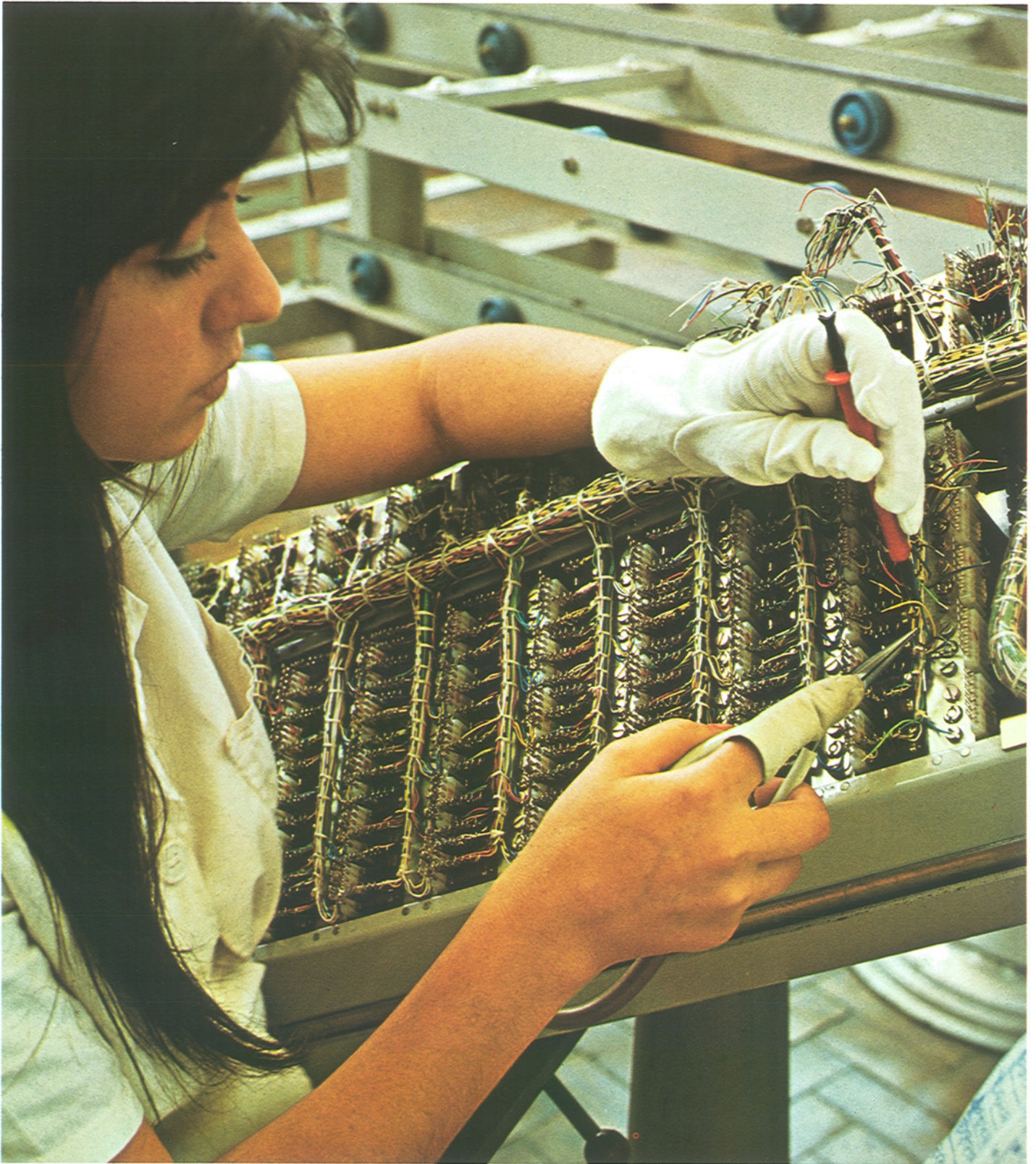
Wiring relay sets at the Ericsson do Brasil factory in São José dos Campos.
