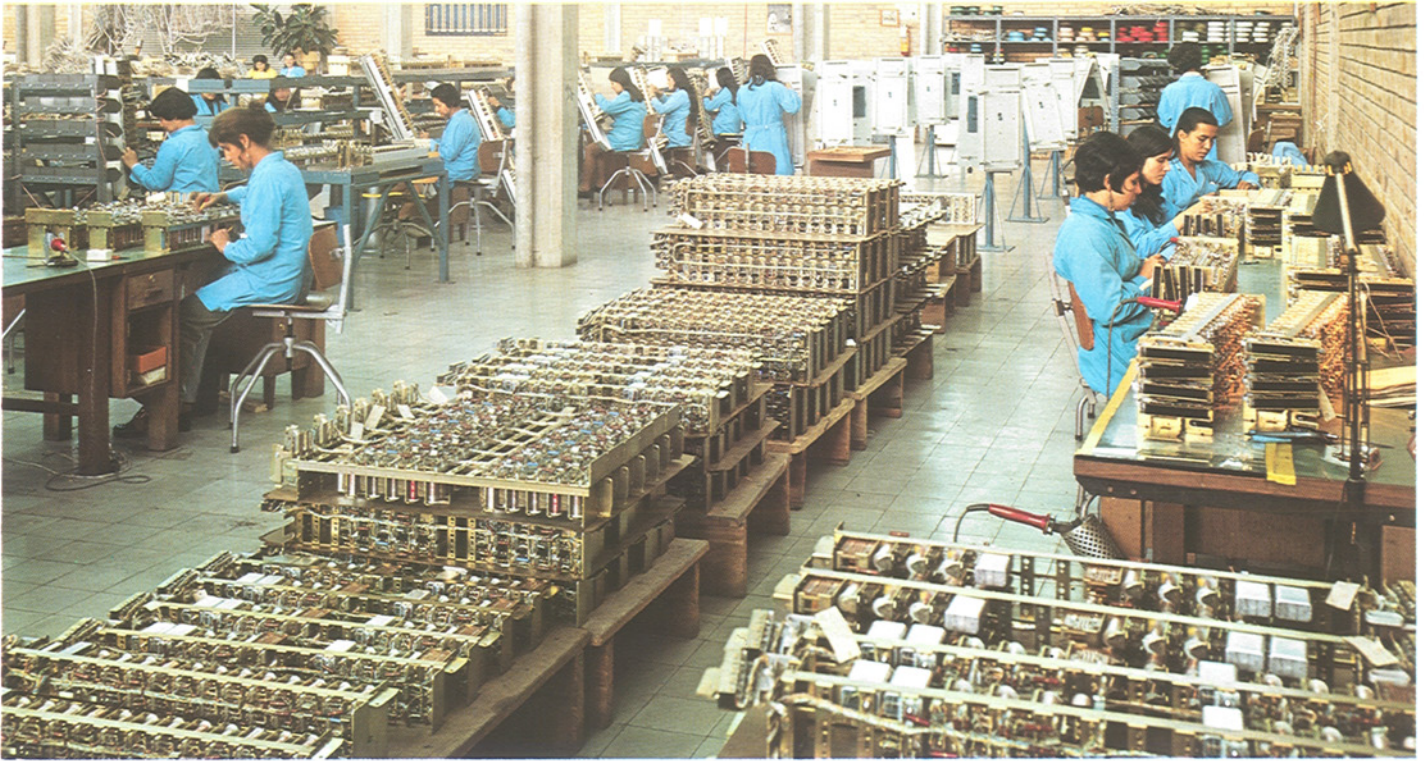
Telephone exchange equipment being manufactured at the Ericsson subsidiary in Colombia, Ericsson de Colombia S.A.
