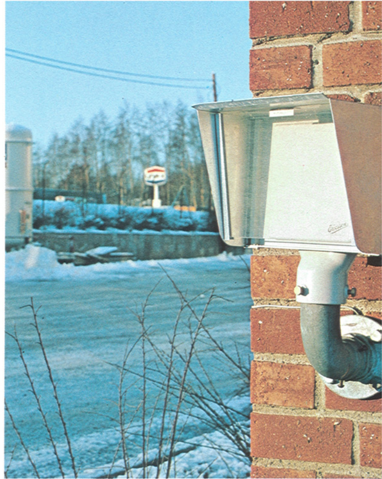
Radar barrier from LM Ericsson Telemateriel AB for outdoor surveillance of industrial zones.
