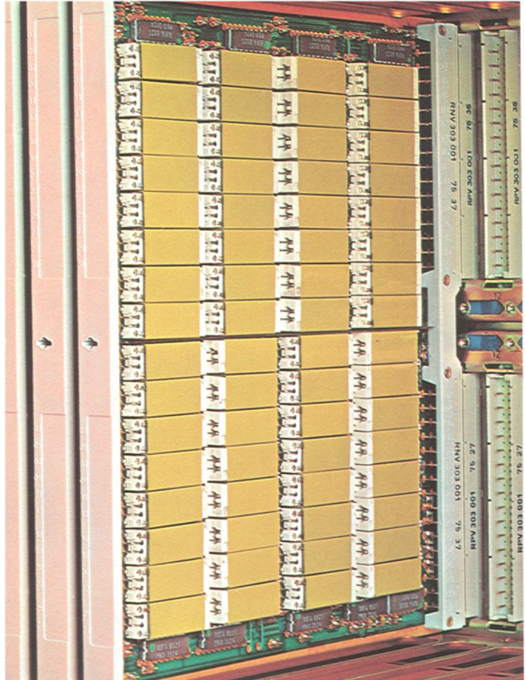
Compact reed switch controlled by integrated electronic circuits and primarily intended for the AXE telephone exchange system.
