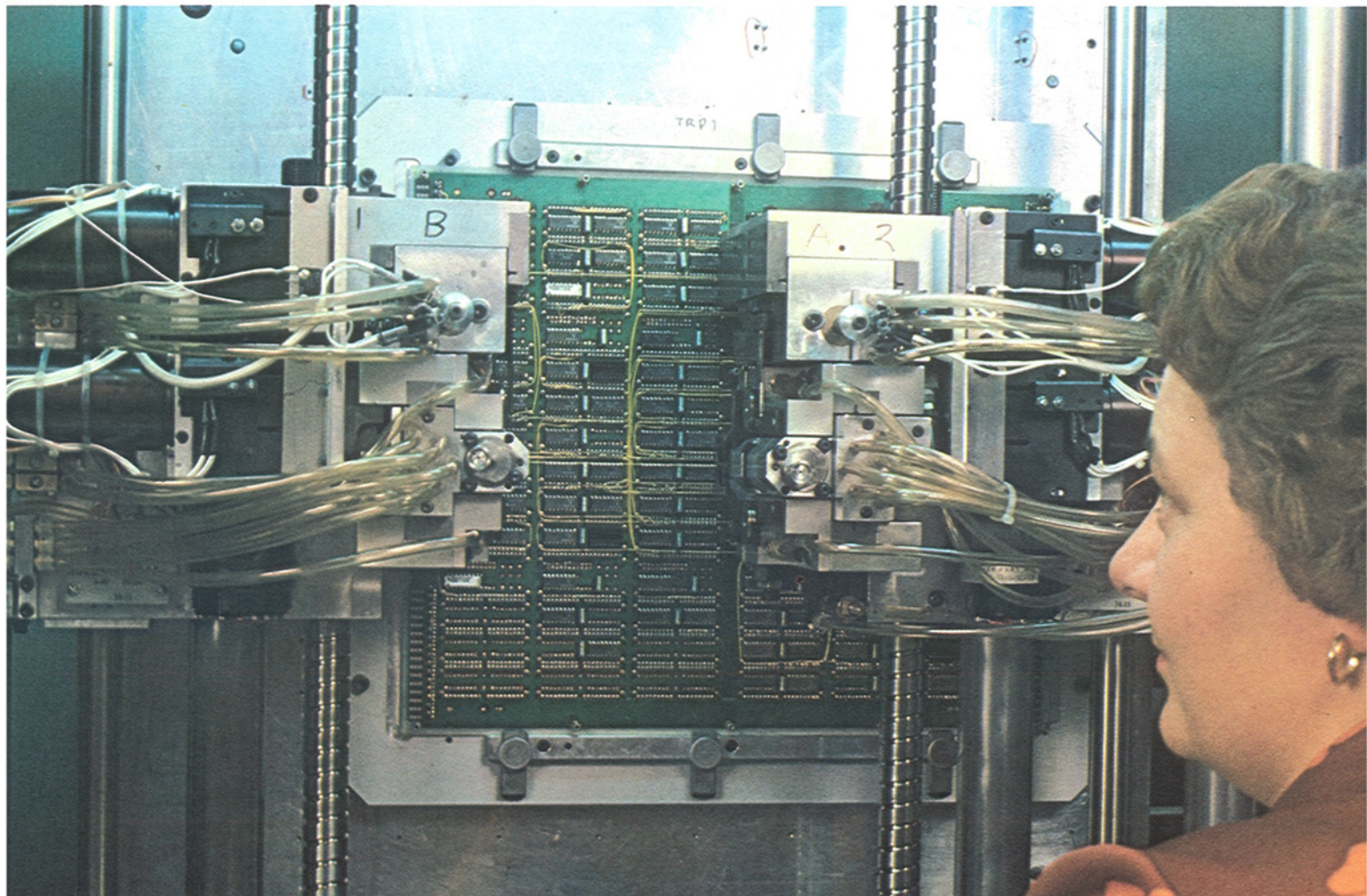
Fully automatic machine for wiring printed circuit cards by means of so-called "lashing," an alternative to soldering.
