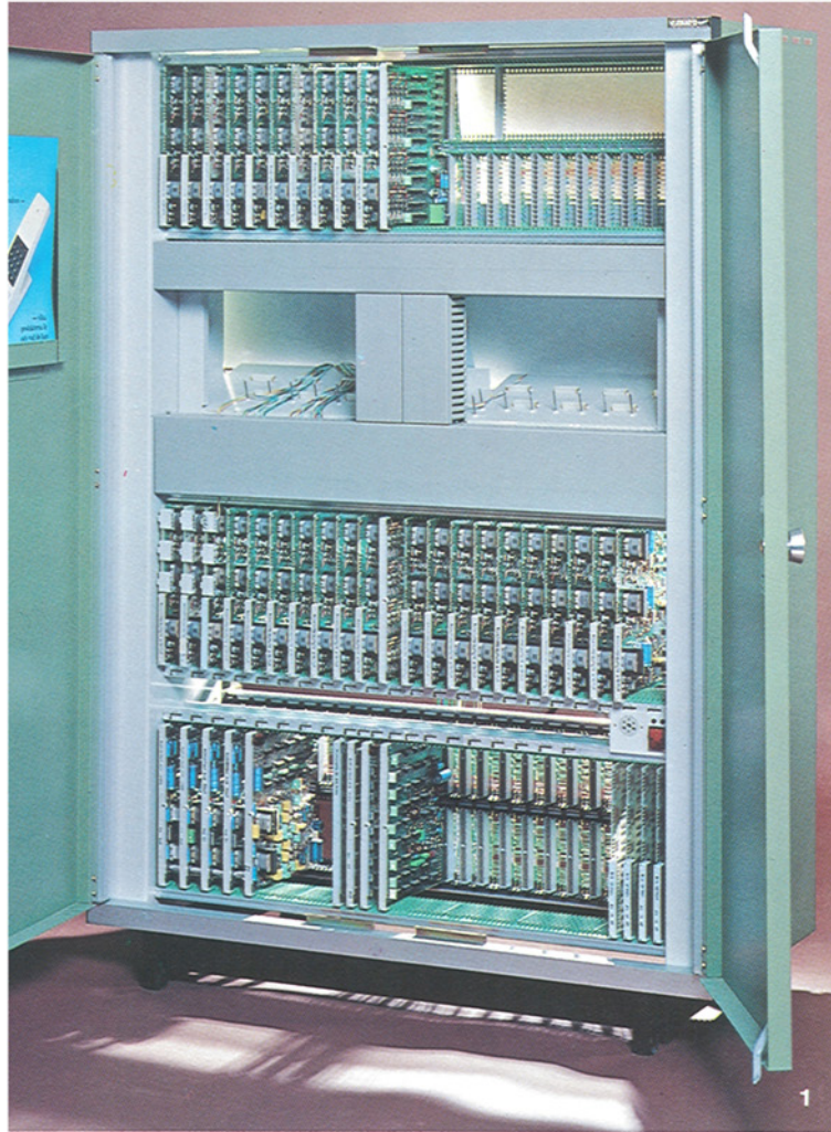
1. ASE 462 electronic intercom exchange produced by LM Ericsson Telemateriel AB.
