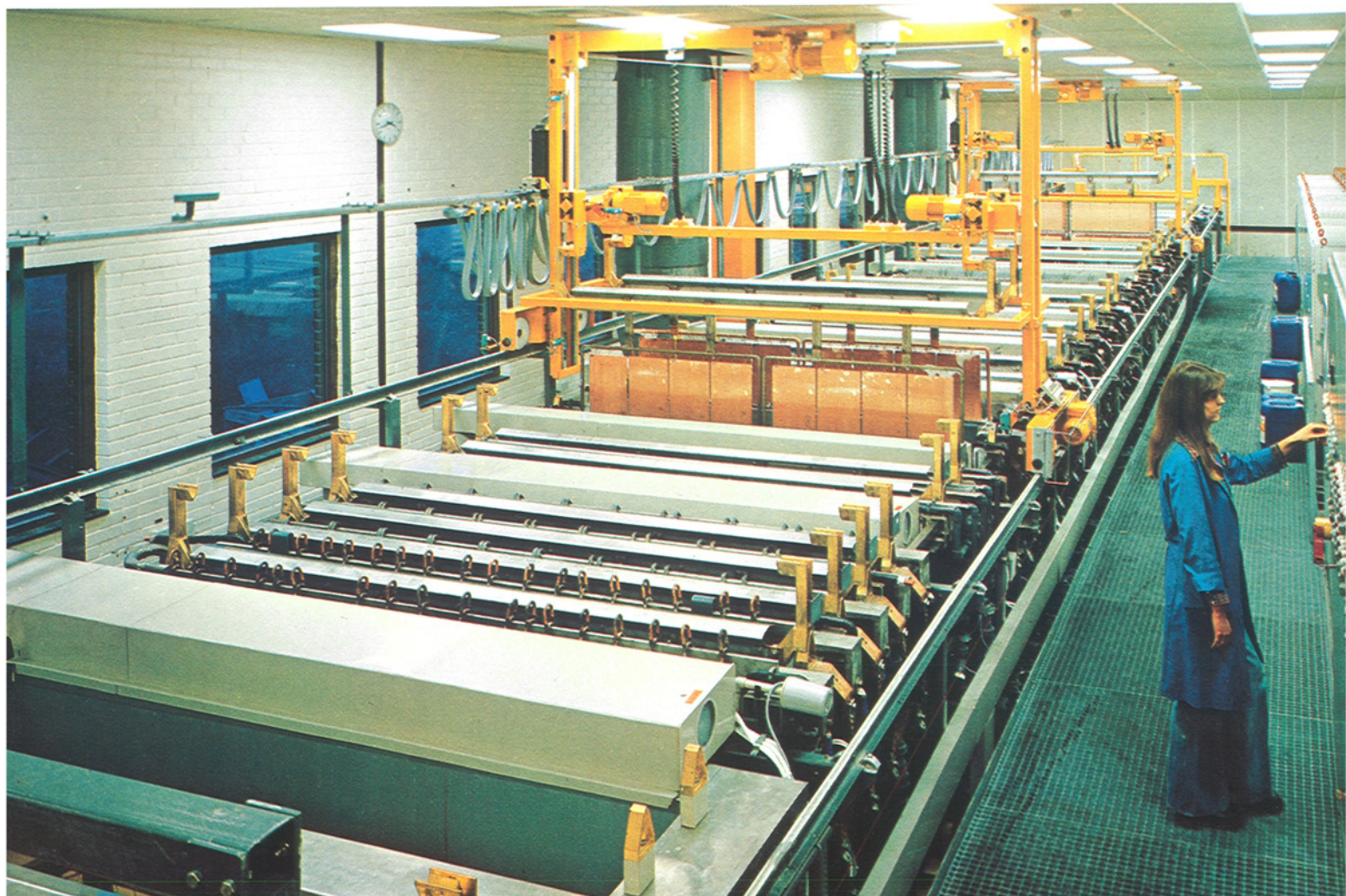
Plating of printed circuit board, using highly automated equipment, in the printed circuit board plant in Norrköping, Sweden.
