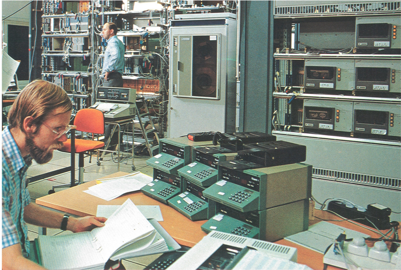
The Nordic data network, which uses Ericsson's AXB 30 switching system, will be placed in service during 1979. Here, the system is being tested in the laboratories of ELLEMTEL Development Company.
