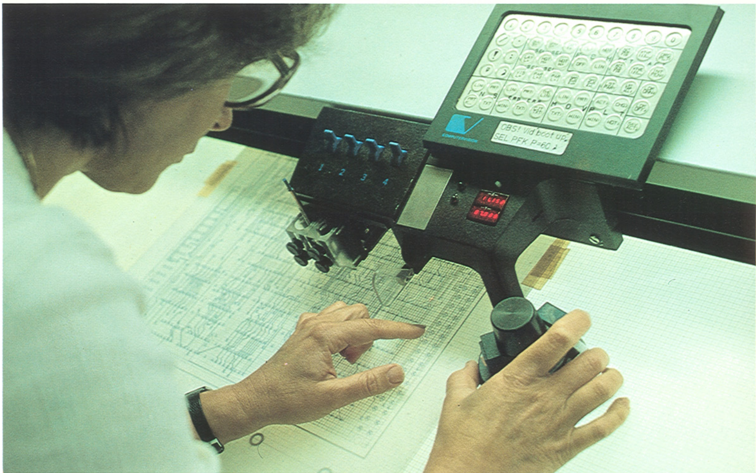
Printed circuit boards are designed at ELLEMTEL with the support of computer programs.
