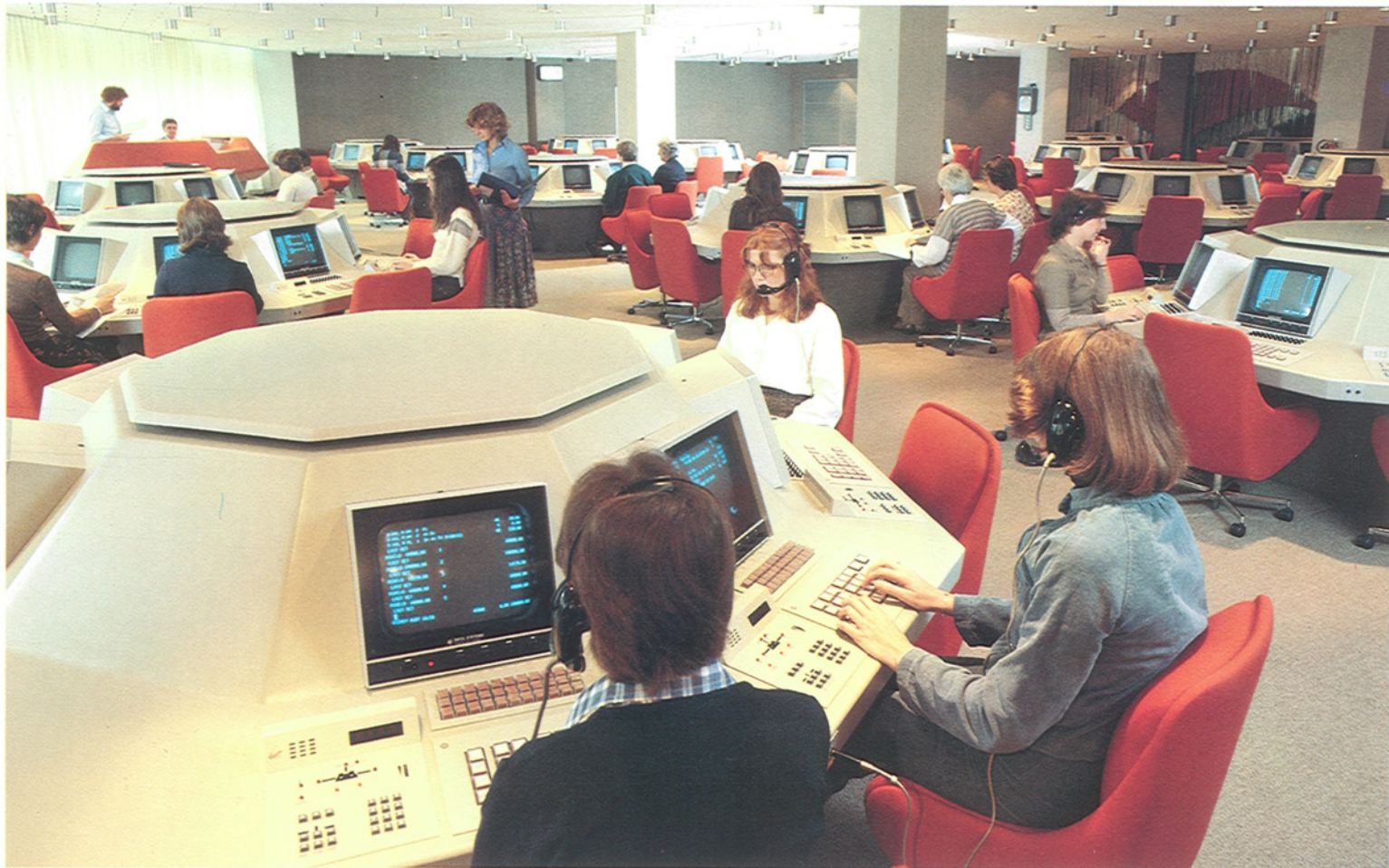
The ASDP 162 is a digital booking and call distribution system for efficient distribution of large volumes of incoming calls.
