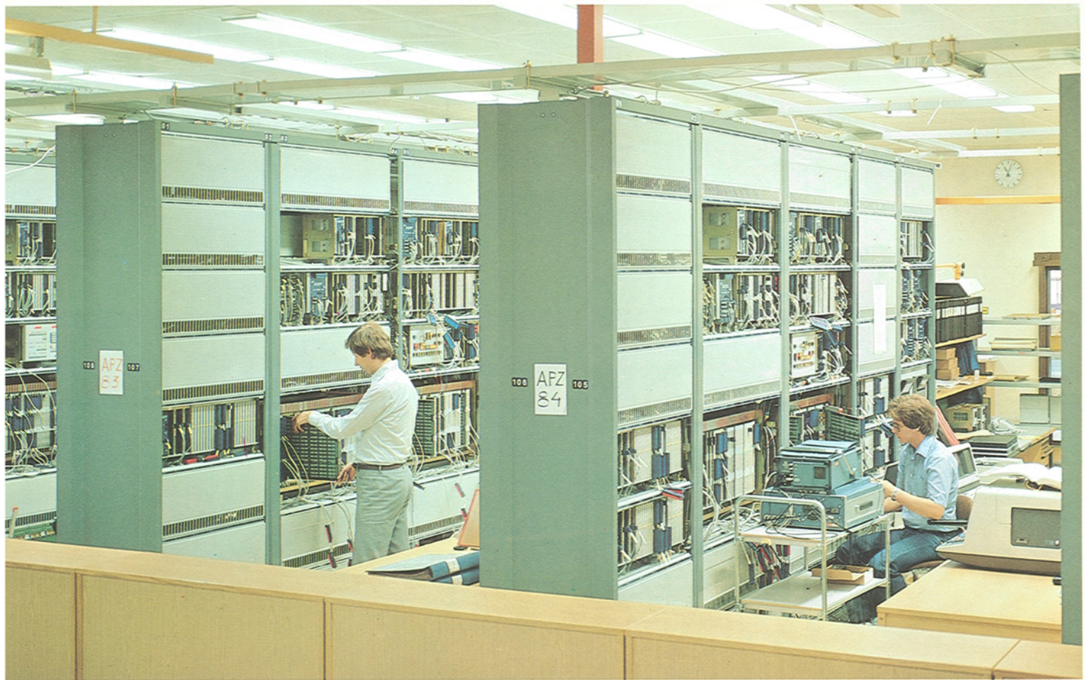
Test stations for final checking of central processors for AXE exchanges at the Group's plant in Älvsjö, near Stockholm.
