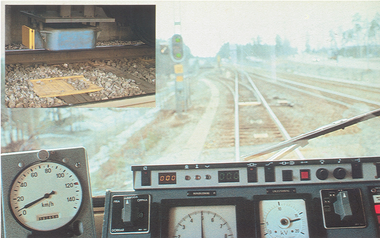
The JZG 700 automatic train control system.
