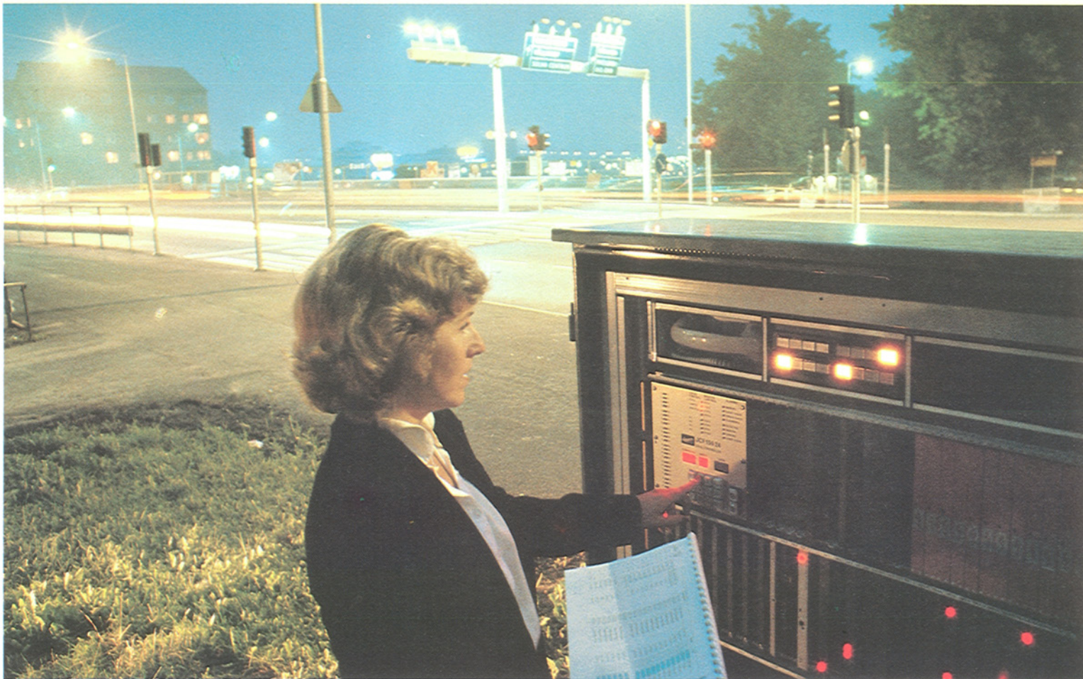
Microcomputer-based control devices for traffic signals are produced by SRA Communications AB.
