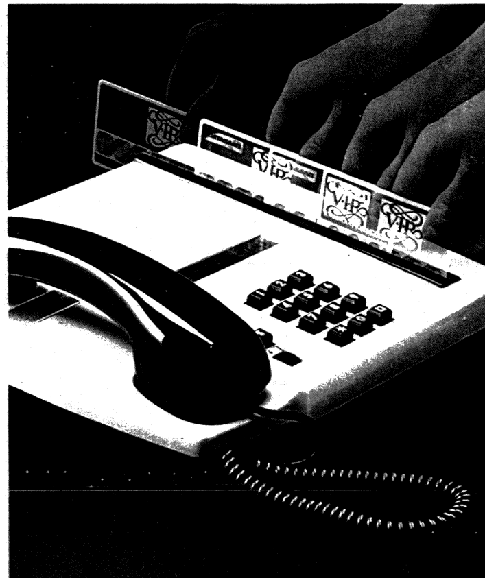
An authorization terminal, connected to the public telephone network, for the automatic recording of bank and credit cards.
