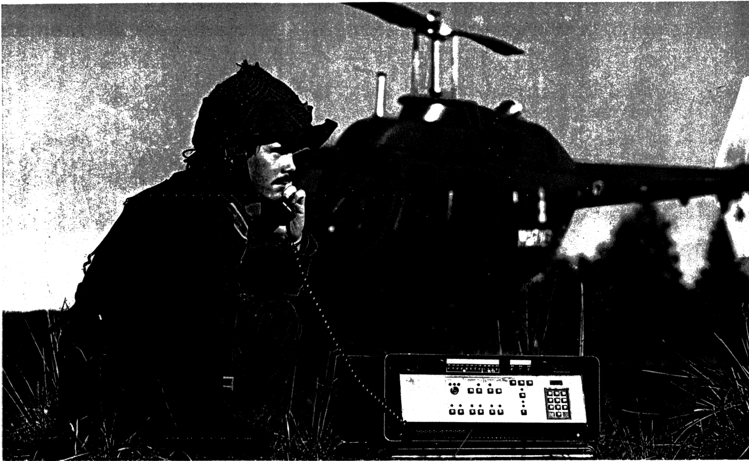
Ericsson's microcomputer-controlled ABM 301 field exchange.
