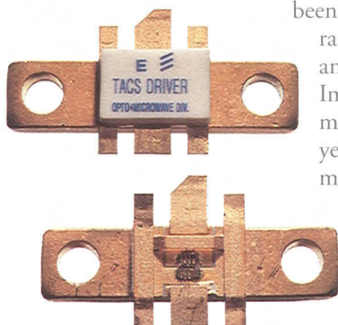
Ericsson Components has developed advanced power transistors for radio base stations.
