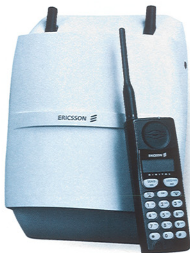
THE RBS 884 ENSURES EFFECTIVE MOBILE COMMUNICATIONS IN DIFFICULT IN-DOOR ENVIRONMENTS.
