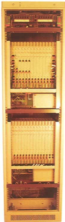
The new generation of AXE switches is extremely compact. Some components have been reduced by as much as 90 percent in size.
