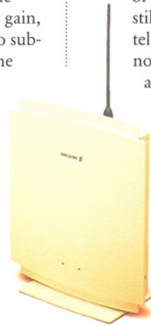
A fixed cellular network uses GSM technology to connect subscribers to the fixed-wire network.
