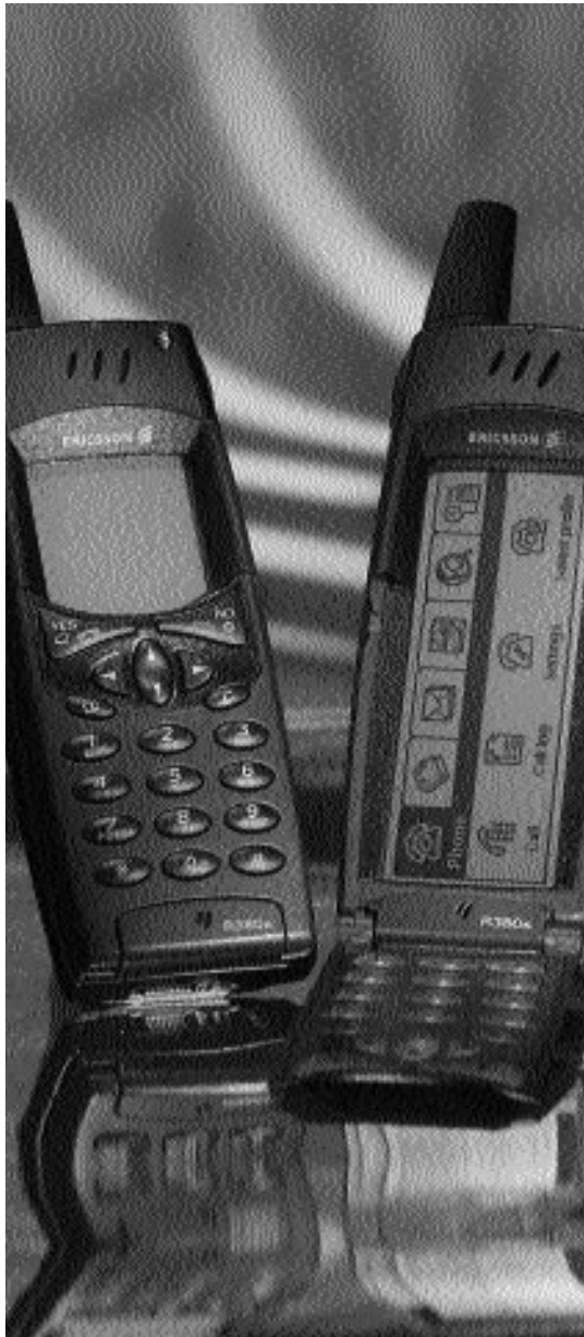
R380, dual-band telephone with built-in PDA, based on EPOC. Communication tool, calendar, built-in modem.
