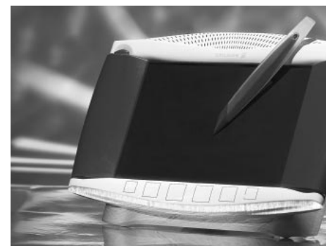
HS210, cordless display phone for home communications. Provides direct access to the Internet and e-mail using Bluetooth technology and a small base station.
