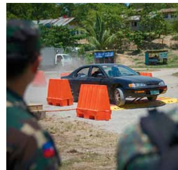
A demonstration of the Pre-emplaced Electric Vehicle Stopper, which uses electrical impulses to disable a vehicle's engine without harming passengers. Booz Allen provided technology development and testing support.
