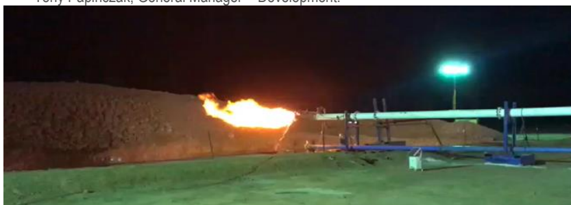
Figure 1 – Flare from Albany 1, which flowed 230,000 scf/d over a 13m interval in the Lake Galilee Sandstone
