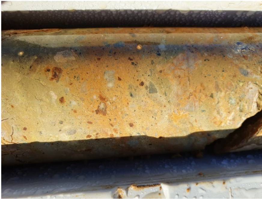
Figure 9: CDX0004 Example of oxidized polymictic breccia
