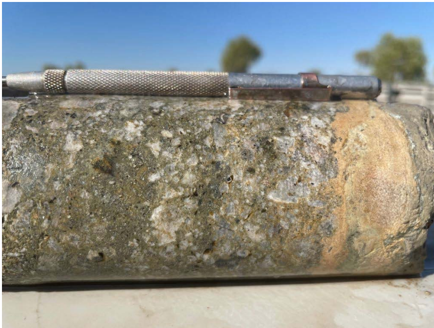
Figure 10: CDX0007 123.5m massive orange monazite forming on lower contact of a primary sulphidic carbonatite breccia within a larger 75m fault breccia
