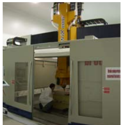
Breton 5 Axis milling machine - One of a handful of large high accuracy machines in Australia
